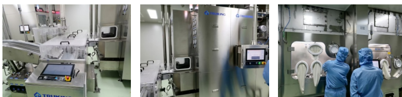
The integrated sterile filling and lyophilization system
